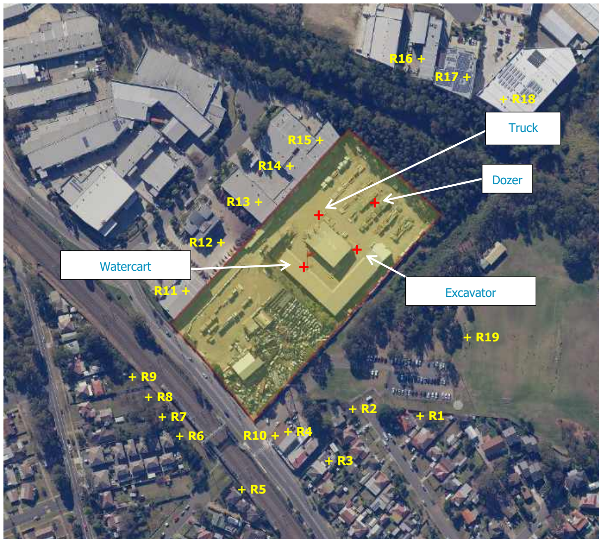
Figure 21 Construction Scenario 1 – General Excavation Works
