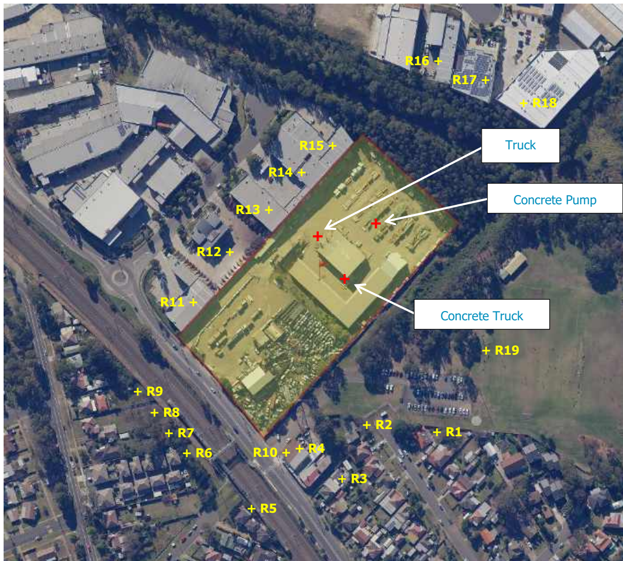
Figure 22 Construction Scenario 2 – Concreting Works
