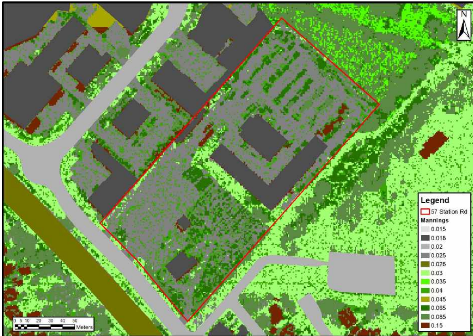
Figure 5 : Existing Landcover (Mannings Roughness)
