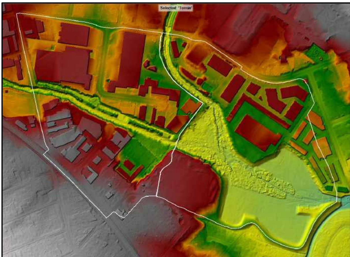
Figure 3 : HEC-RAS 6 model Terrain Grid with 2D Flow Area Extent (from RAS Mapper)
